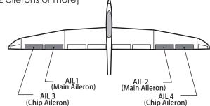
Select [Aileron differential] at the model menu and call the setup screen shown below.
