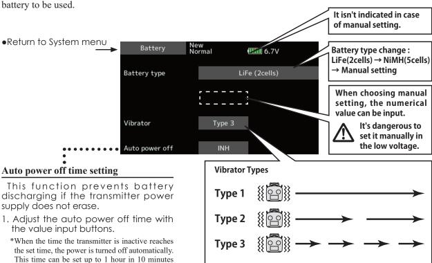
\*An audible alarm is sounded from 3 minutes before auto power off. When a stick or switch is operated, the alarm is cleared.
