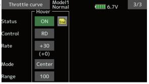
The Throttle Hover function trims the throttle near the hovering point. Normally, use it with hovering conditions. Changes in rotor speed accompanying changes in the temperature, humidity, and other flight conditions can be trimmed. Adjust the throttle so that rotor rotation is most stable. More delicate trimming is also possible by using this function along with the Hover Pitch function.
