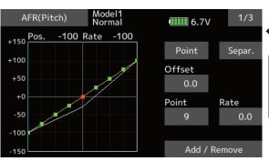
Point curve type is 9 points (initial), but for simple use, 4~5 points are sufficient.
