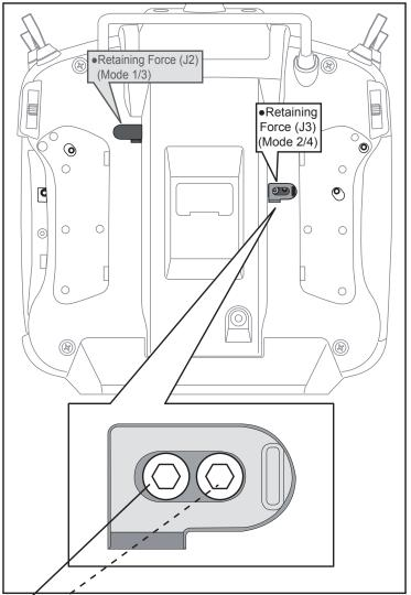
\*In the Mode 1/3, arrangement of a screw is opposite.
