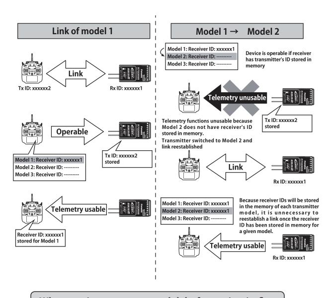
When setting up a new model, before using it, first establish a link with the receiver that will be used with it.
