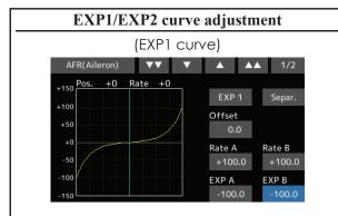
Using the EXP1 curve is effective in smoothing starting of the ailerons, elevator, rudder, etc.
