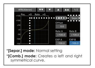
Point curves or spline curves of up to 11/17 points can be used. (Initial value: 7/9 points) **The set points can be freely increased**, decreased, and offset.
