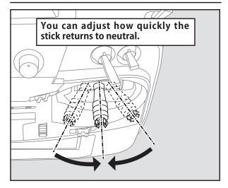
The tension of the self-return type stick lever can be adjusted.
