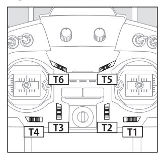
This transmitter is equipped with 6 digital trims. Each time you press a trim button, the trim position moves one step. If you continue pressing it, the trim position starts to move faster. In addition, when the trim position returns to the center, the tone will change. You can always monitor trim positions by referencing the LCD screen.
