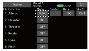
"NORM": The model is controlled by signals from the student transmitter.
