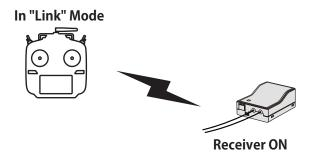
8. If linking fails, an error message is displayed. Bring the transmitter closer to the receiver and repeat the procedure above from Step 2. 9. ACT will be chosen if telemetry is used. It is INH when not using it.
