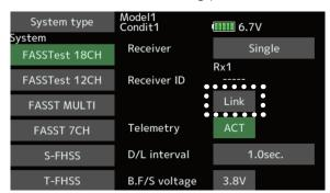
7. When the transmitter starts to chime, power on the receiver. The receiver should link to the transmitter within about 1 second.
