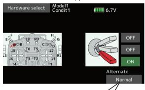
Normal or Alternate: Alternate switching mode is available depending on mixing function.
