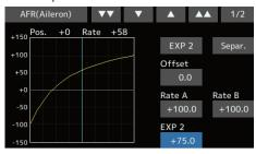
Using the EXP2 curve is effective in engine rise and other engine control.
