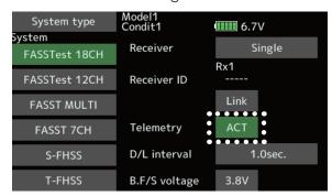
10. When a telemetry function is enabled, the receiving interval (down-link interval) of sensor data can be changed. If a D/L interval is increased, the response of the sensor data display becomes slower, but stick response will improve.
