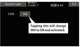
2 Tap the "CRSF" button to [ON]. A signal conforming to the CRSF standard is output from the S.BUS setting connector (S.I/F) of the transmitter.
