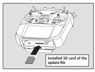
6. Turn on the transmitter power while pressing down the "HOME/EXIT" button. The update screen appears on the LCD display of your T18SZ and the software update is started.
