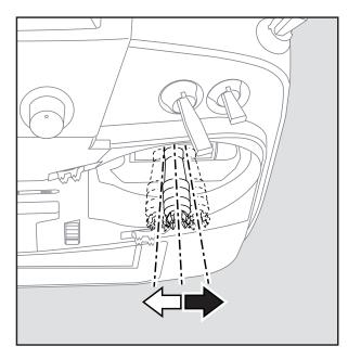
Use the attached 1.5mm hexagonal wrench (inside stylus) to turn the screw clockwise to adjust the stick outwards, or counter-clockwise to tilt it inward.
