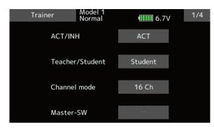
Note: In "student mode", only the teacher side can turn on and off the power to the student's transmitter. Keep the power switch always at off position.
