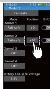
Fail-Safe position setting While holding the wheel or trigger, tap the Fail-Safe position button.
