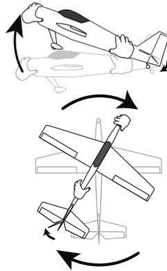
Tilt the airplane to the left on the ground and check that the rudder operate to the right. (In the case of rudder control)
