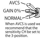
Refer to the transmitter instruction manual and set the end point. When AVCS is used, setting the 3-positions switch to the sensitivity CH (there are types which cannot be set by transmitter) and setting it as shown above is recommended. In the case of a 2-positions switch, inhibiting the gyro at 0% sensitivity such as NORMAL mode and sensitivity 0% and AVCS mode and 0% sensitivity is safe.
