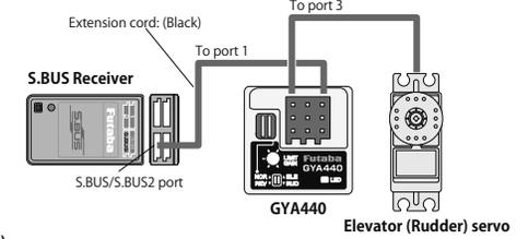
At S.BUS/S.BUS2 operation, the channels are fixed as shown in the table below. Match the transmitter channels to these.
