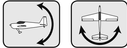
Thank you for purchasing the GYA440 airplane gyro. Compact and lightweight, the GYA440 is designed to control the elevators (pitch axis) or rudder (yaw axis). Features include simple set-up and S.BUS/S.BUS2 connectivity.
