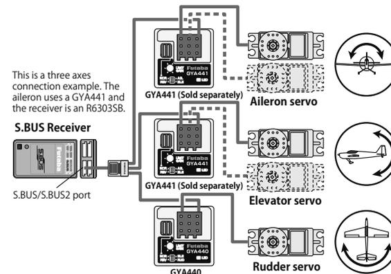
S.BUS connectivity minimizes wiring. The GYA440 and GYA441 can be connected by one 3-way hub. The aileron, elevator, and rudder servos are output from the gyro. Standards servos can also be used. When an R6303SB is used the CH switching mode is set to group 7. The normal group 7 CH outputs are CH3, CH11, and CH12. CH3 is the throttle channel and CH11/CH12 are spare channels.
