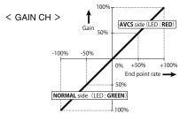
3CH (GAIN CH) is set up with reference to the manual of a transmitter. A neutral becomes GAIN 0%. It is divided into AVCS side and NORMAL side. Check using the GYC440's LED.
