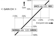
3CH (GAIN CH) is set up with reference to the manual of a transmitter. Neutral position becomes GAIN 0%. It is divided into AVCS side and NORMAL side. Check using the GYD450's LED.
