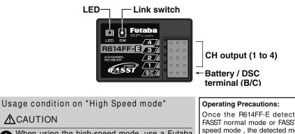
**D** When using the high-speed mode, use a Futaba digital servo (including brushless servo). Analog servos cannot be used.
