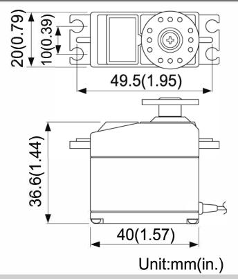
•Use the horn set screw supplied with the servo. (Screw size: 3x8mm) The servo horn can be used the only 3mm in diameter of the hole center.
