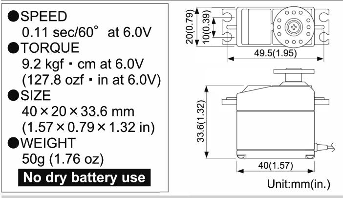
•Use the horn set screw supplied with the servo. (Screw size: 3x8mm) The servo horn can be used the only 3mm in diameter of the hole center.
