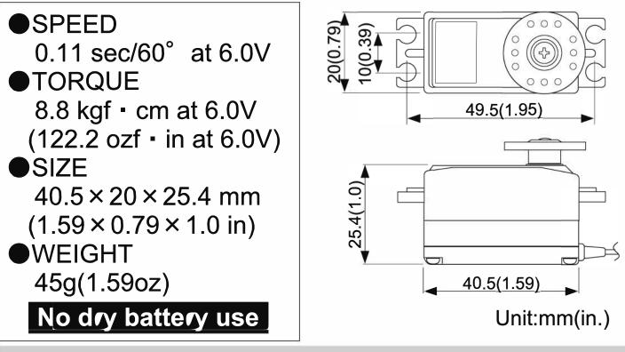
•Use the horn set screw supplied with the servo. (Screw size: 3x8mm) The servo horn can be used the only 3mm in diameter of the hole center.
