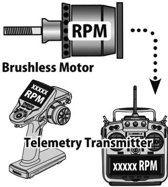
The RPM of a brushless motor can be viewed on your transmitter without removing the motor's magnet using only a wiring connection (soldering is necessary).
