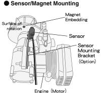
The distance between the sensor and the magnet must be 1-2mm.
