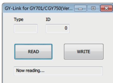
5). Once the reading process is complete, the box shows model type and ID number. When you have Read error message or box does not show the ID number, make sure the wire connection and power supply and retry the reading process again.
