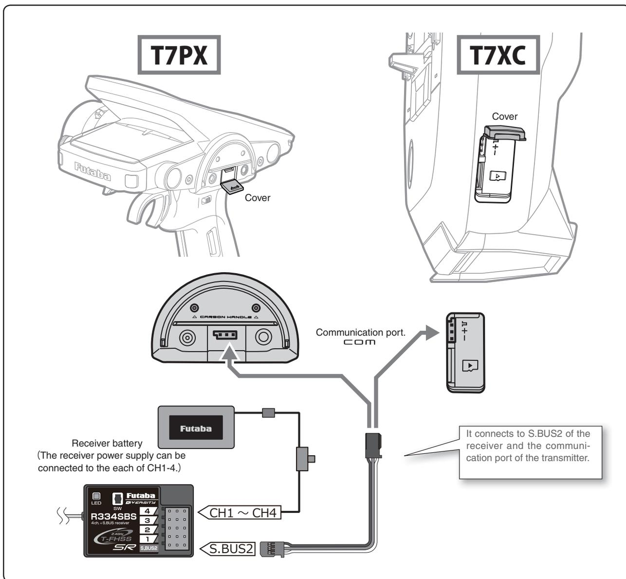
Turn on the DSP or PWR switch of T7PX/T7XC and display the receiver update screen.
