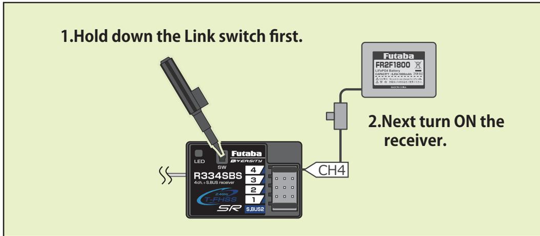
5. Once the LED confirms by flashing red once, release the Link switch and press again.
