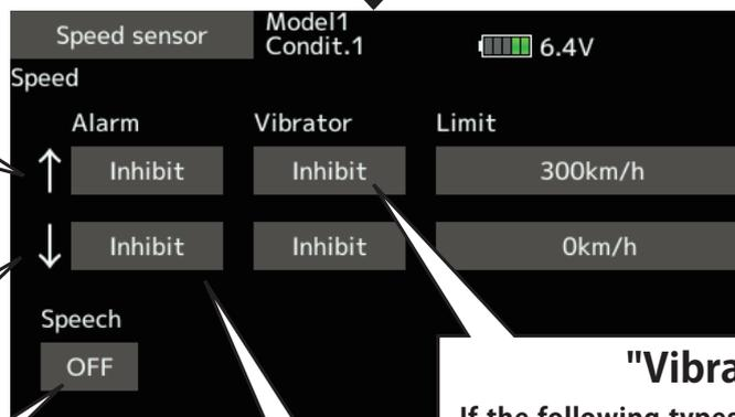
A setup of the speed on which the alarm operates.
