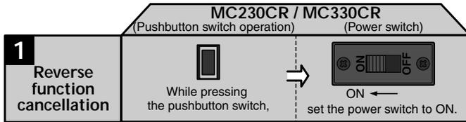
\* When desired, you can enable the cancelled reverse function by repeating the operation shown at the left. (The reverse function is switched alternately.)
