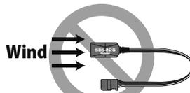
Do not install in a location where the wind/air flow can hit the sensor.
