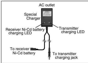
Before use, always charge a new battery or a battery that has not been used for a long time. We also recommend that the battery be charged about once a month even when not used for a long time.
