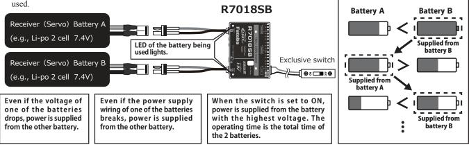
This receiver employs an electronic switching (current is controlled by an FET circuit) system. When the exclusive switch is set to ON or is pulled, the power is turned on. Switches other than the exclusive switch cannot be used. In addition, since a very small current flows even when the power is off, always disconnect the battery from the connector when the receiver is not in use.
