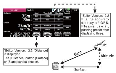
■ GPS (altitude) and GPS (variometer) setting screen This screen displays the altitude, variometer, and air pressure. When [Preset] of [Reference Point (Altitude)] is touched, the altitude measurement reference altitude is initialized.
