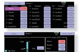
Adjust the direction of operation of the gyro. (Gyro side function)
