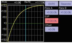
Using the EXP2 curve is helpful in engine rise and other engine control.
