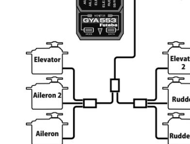
Thank you for purchasing the GYA553 airplane gyro. Compact and lightweight, the GYA553 is designed to control the ailerons (roll axis), elevators (pitch axis) and rudders (yaw axis). In addition, the GYA553 is equipped with a recovery mode to avoid danger. Features include simple set-up and S.BUS/S.BUS2 connectivity.
