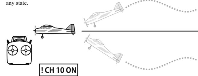
Turn off the recovery switch when return to level flight. It will be a normal flight. Maneuvering is possible even when the recovery switch is ON, but the operation differs as follows.
