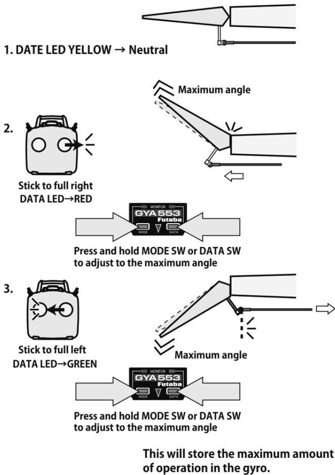
If the servo operates more than the maximum operating position, the servo and linkage will be overloaded and may be damaged. To prevent this, be sure to set this limit on all servos at the time of initial setting.
