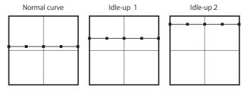
In governor mode, set the throttle curve to a horizontal straight line. Set the value according to the rotor speed
