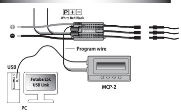
Connect the ESC, Program box and PC according to the picture.
