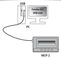
Sometimes the firmware of Program box should be updated because the functions of ESC are improved continuously.
