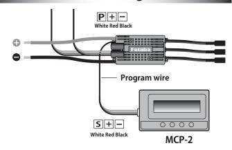
\* The figure is an example of MC-980H/A. For the ESC connection port, refer to the respective ESC instruction manual.
