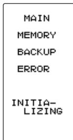
If the data in the transmitter is not transferred normally when the power is turned on, an audible alarm will sound and "MAIN MEMORY BACKUP ERROR" will be displayed on the LCD. When a memory error is generated, request repair from the Futaba Service Center.
