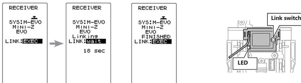
Touch the [END] button on the link screen of the transmitter to cancel the link mode. Please check the operation.
