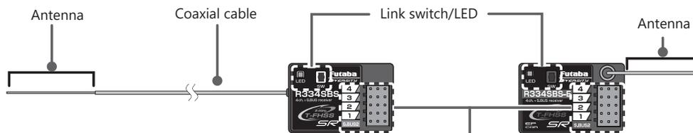
\*The receiver power supply can be connected to the S.BUS2 connector or each of CH1-4.
