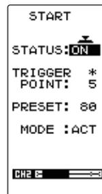
The throttle servo moves to the "PRESET" position and the status display is "ON".
