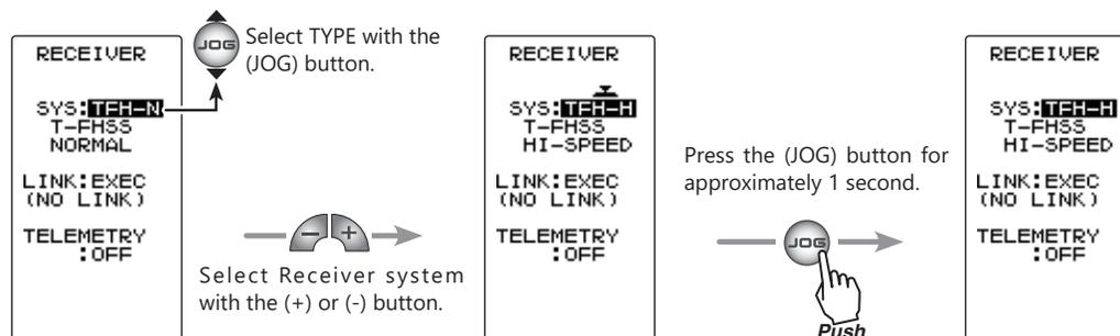
\*When using an S-FHSS system ("SFH") receiver (R2104GF, R204GF-E, etc.), after reaching this point set the transmitter power switch to OFF and go to ["Receivers Other Than T-FHSS" on page 32.](#)
