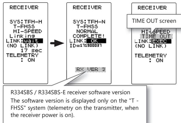
\*The T4PM PLUS and a telemetry type T-FHSS receiver (R334SBS, etc.) mutually memorize the combined ID linked last at each model memory.
