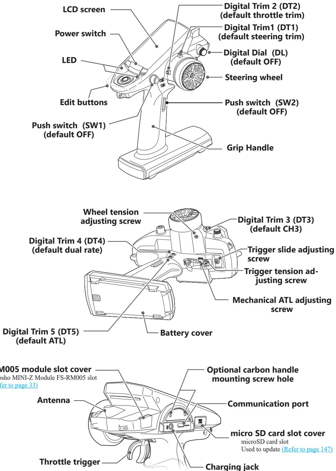
\*The switches, dial, and trimmers in the figure are shown in the initial setting position.
