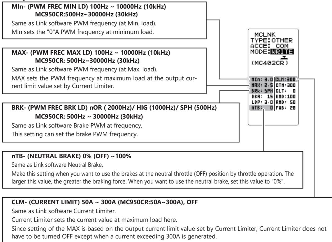
"Min", which sets the frequency when the load is small, is set to the high frequency side (large value) when extension is desired after straightaways and curves.
