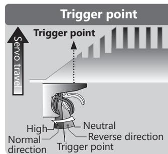
Select the setting item "TYPE" by moving the (JOG) button up or down. Use the (+) or (-) button to set the operating range.
