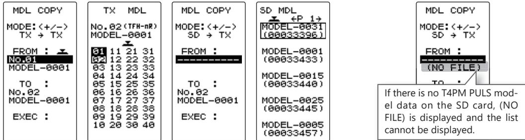
Select the copy destination model with the (JOG) button up / down or left / right operation, and press the (JOG) button. Return to the copy screen.
