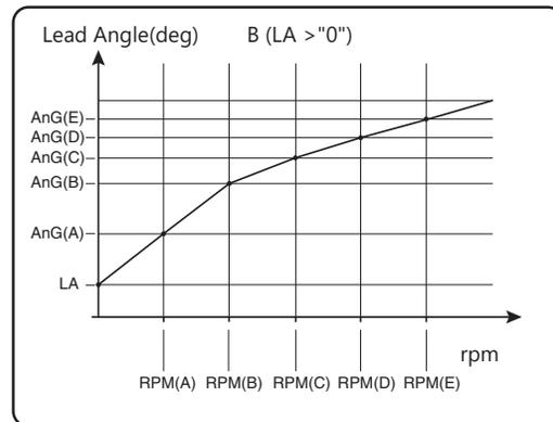
When using in races in which the lead angle setting function is inhibited by the ESC, set LAU (LEAD ANGLE USE) to OFF. The LAU setting has priority over TBM-(TURBO MODE). If LAU is set to "OFF", the lead angle setting function can be turned off even if TBM is set to "LV1" or "LV2". The MC940,960CR shows that the lead angle setting function is OFF ("0" timing) by blinking a LED.
