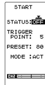
The Start function is automatically deactivated and the set returns to normal throttle trigger operation. The status display is "OFF".
