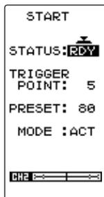
Operate (or pass) the throttle trigger from the status display "RDY" to the trigger position.
