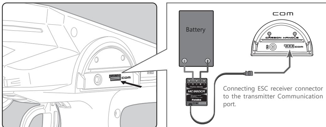
Display "MC LINK" screen using the following method:
