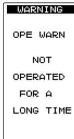
If the T4PM PLUS is not operated for 10 minutes, an audible alarm is sounded and "OPE WARN" is displayed on the screen. The audible alarm stops when the steering wheel, throttle trigger, and any dial, switch, or edit button is operated. If you are not going to use the transmitter, turn the power off. (Setting can be reset at the system menu on [page 44](#).)
