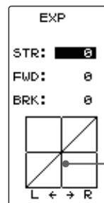
Vertical cursor moves in step with steering wheel operation.
