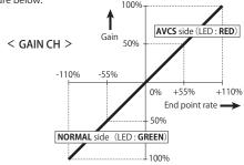
3CH (GAIN CH) is set up with reference to the transmitter manual. Neutral position becomes GAIN 0%. It is divided into AVCS side and NORMAL side. Refer to the GYC470's LED.
