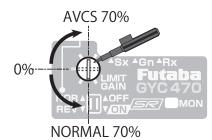
Receiver ON → The GYC470 requires 3-5 seconds to initialize when the power is turned on. Do not move the car and do not move the steering wheel during this initialization or the gyro may not initialize properly. Once the initialization process has been completed, the steering servo will move slightly several times, indicating that the GYC470 is now ready for use. If neutral has shifted, LED will blink orange. In that case, it reboots.
