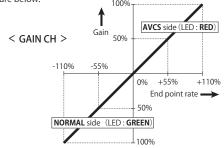
3CH (GAIN CH) is set up with reference to the manual of a transmitter. Neutral position becomes GAIN 0%. It is divided into AVCS side and NORMAL side. Check using the GYD470's LED.
