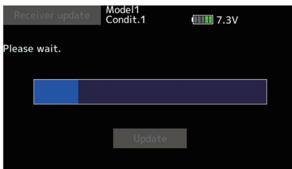
15. During the update, the update bar graph on the transmitter progresses and the green LED on the R7208SB/R7308SB flickers.
