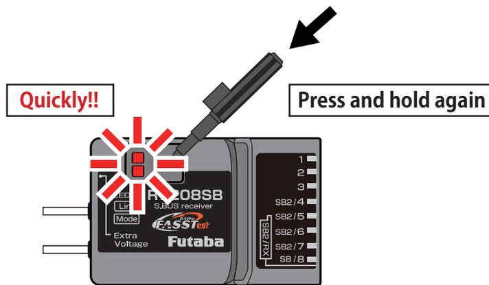
12. Release the switch when the solid orange.
