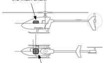
• The roll axis must be parallel to the tail boom and the pitch axis must be perpendicular to the side frame.
