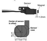
☐ The center of the sensor is different from the center of the sensor case so be careful when mounting the sensor.
