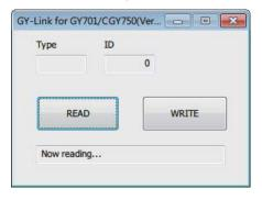
5).Once the reading process is complete, the box shows model type and ID number. When you have Read error message or box does not show the ID number, make sure the wire connection and power supply and retry the reading process again.
