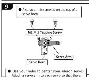
is parallel with the hinge line when the servo is centered. Install the arms so that they point
