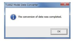
5.3. Depending upon the source and destination transmitter models, a warning dialog might appear. Read the information in the dialog box prior to clicking the "OK" button. Additionally, we suggest that you check the operation of the model prior to flight.
