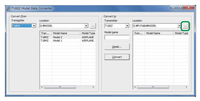
3.2. Click on the "Model name" text box. Using the PC's keyboard, enter a new name for the model. Please note: this will be the name displayed in the "Model name" columns of the "Convert to" group box when the data is converted.
