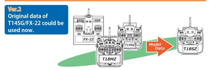
The T18SZ Model Data Converter is a software that converts model data of T18MZ/T14SG/FX-22 to that for T18SZ. The software cannot convert model data that made by other transmitters such as T14MZ etc. Thus please still use the existing converter - Futaba Model Data Converter Ver.1.0.4, if you want to convert model data of T14MZ/FX-40/T12Z/T12FG/FX-30.
