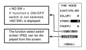
If the power switch is turned on while the neutral brake switch is on, an audible alarm will be heard. Immediately set the neutral brake switch to OFF.
