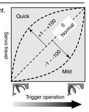
2 Brake Exponential Adjustment Select the setting item "\*EXPB" by (UP) or (DN) button. Use the plus (+) button to adjust for a faster brake response or use the minus (-) button for a slower or milder brake response.
