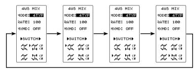
"4TYP": Front side only, reverse phase, same phase, and rear side only switching
