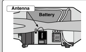
Install the receiver as far away as possible from the battery, motor controller, motor, silicon cord and other noise sources. Keep it away from the antenna wire, in particular.
