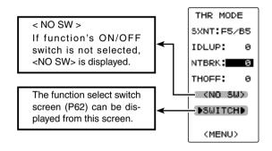
If the power switch is turned on while the throttle-off switch is on, an audible alarm will be heard. Immediately set the neutral brake switch to OFF.
