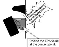
Adjust the steering servo so that unreasonable force is not applied to the servo by the chassis at maximum servo travel.
