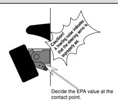
Adjust the steering servo so that unreasonable force is not applied to the servo by the chassis at maximum servo travel.
