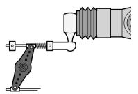
Adjust the throttle servo so that unreasonable force is not applied when the engine carburetor is fully open, fully closed, and the brakes are applied fully.
