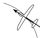
Nose points inside circle: too much coupling or differential. Reduce one or both.
