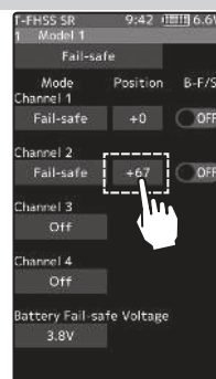
Fail-Safe position setting While holding the stick, tap the Fail-Safe position button.
