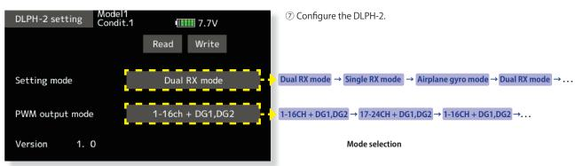
\*When setting mode is set to [Airplane gyro mode], PWM output mode is fixed to [1-16CH + DG1,DG2]. \* T16IZS cannot operate after 17ch. (8) Tap [Write]. → DLPH-2 settings will be changed.
