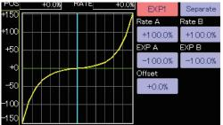
• Using the EXP1 curve is helpful in smoothening starting of the ailerons, elevators, rudder, etc.
