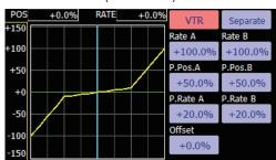
• Setting is fast if left, right, up, and down are first decided in the Combined mode and the mode is then switched to the Separate mode.
