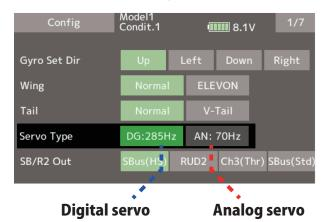
Select the servo type according to the servo to be used.
