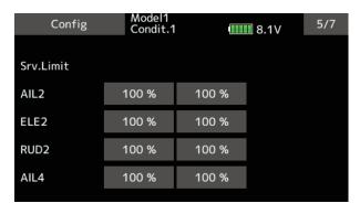
If the SB/R2 port output is set to "S.BUS(HS)" or "S.BUS(STD)", the setting menu will display AIL3 and AIL4 setting items.
