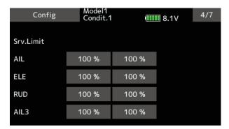
This is the limit setting for each servo. The position of the maximum operation is read into the gyro in the first setting.
