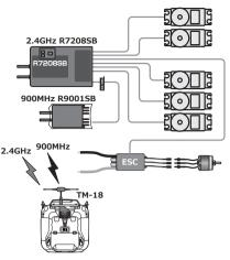
By using Futaba AdRCSS 900MHz and Futaba 2.4GHz system together will provide the better secure RF link.
