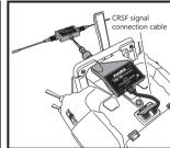
\* In the case of T32MZ, attach the included mounting parts and double-sided tape as shown in the figure.
