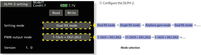
\*When setting mode is set to [Airplane gyro mode], PWM output mode is fixed to [1-16CH + DG1,DG2].
