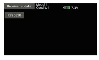
® The update screen is displayed. Connect the receiver or gyro to be updated to the S.I/F connector of the transmitter, prepare for update, and then tap the [Update] button.
