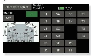
(§) The operated switch is selected. Sets the current switch position to **ON**. Operating the switch changes the **ON** position.
