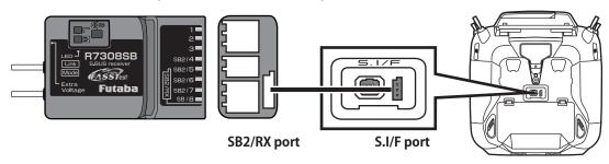
② Turn on the power switch while pressing the **U.MENU/MON** button on the transmitter.
