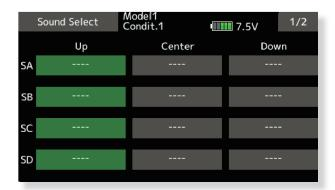
■ Tap on the desired sound to add the requested sound in the previously selected switch position. (It will demo the sound once pressed)
