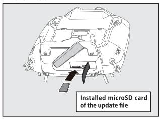
6. Turn on the transmitter power while pressing down the "HOME/EXIT" button. The update screen appears on the LCD display of your T16IZ SUPER and the software update is started.
