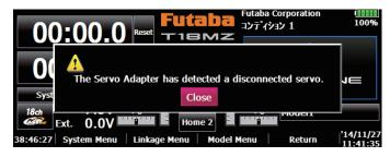
This screen appears and an alarm sounds to indicate a servo connection error.
