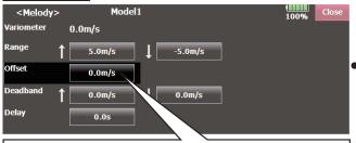
This is the changing point of climb and sink. When the variometer is greater than this value, Vario Melody is climb type. When the variometer is less than this value, Vario Melody is sink type.
