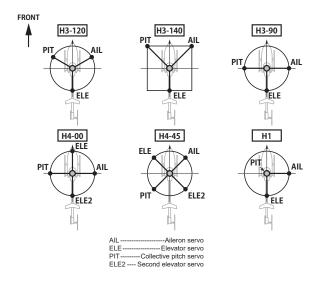
Your transmitter should be reset to the default settings and the swash plate type selected with the transmitter should be set to "H1" or single servo mode. All CCPM mixing is set up and handled in the CGY, and the transmitter functions should not be used. Before starting model set-up, be sure that all dual rates, pitch curve, and endpoint values are set to 100/100.
