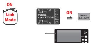
3. After powering on the receiver, please allow for approximately two seconds for the binding/linking to occur.
