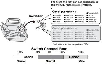
Function Menu of your transmitter (DG1). Assigning DG1 to a switch or flight mode allows the use of two separate values for the condition selectable parameters.
