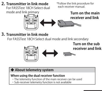
\*The main receiver must receive signals once and switch to the sub receiver only after the gyro initialization is completed.
