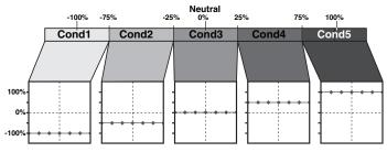
• If you set a condition switch channel, using the AFR function on that channel set a flat point curve for each flight condition. Then you can utilize all 5 flights
