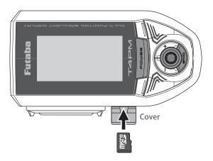
6. Turn on the transmitter power while pressing down the "END" button. The update screen appears on the LCD display of your T4PM and the software update is started.
