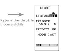
The Start function is automatically deactivated and the set returns to normal throttle trigger operation. The status display is "OFF".
