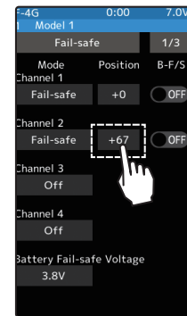
Fail-Safe position setting While holding the wheel or trigger, tap the Fail-Safe position button.
